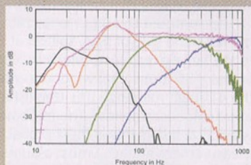
Fig.3 Krell Resolution 1, nearfield responses of the midrange unit (blue), upper woofer (green), lower woofers (red), and ports (black), with the complex sum of the nearfield responses (magenta), weighted in the ratio of the square roots of the radiating areas.
